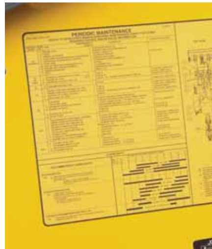
Convenient lube and periodic maintenance chart ensures that nothing gets overlooked. Synthetic bushings in the loader linkage and extendable dipperstick eliminate numerous grease zerks.
